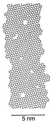
Figure 43. Drawing of a model graphene layer in a CF showing vacancy defects. [221] Reproduced with permission from Maney Publishing.
